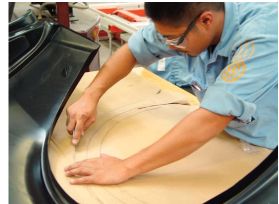
ABRP student creates a template for composite repair.
