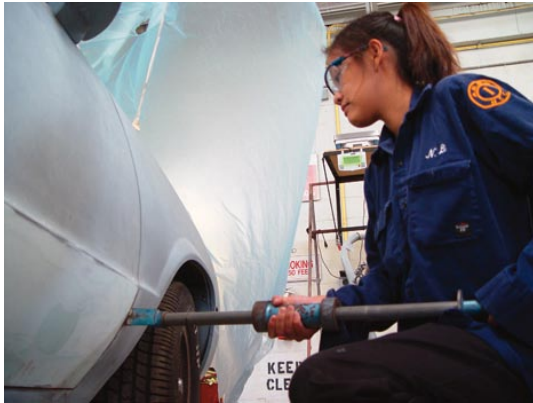
ABRP student uses tool to repair a dent.
