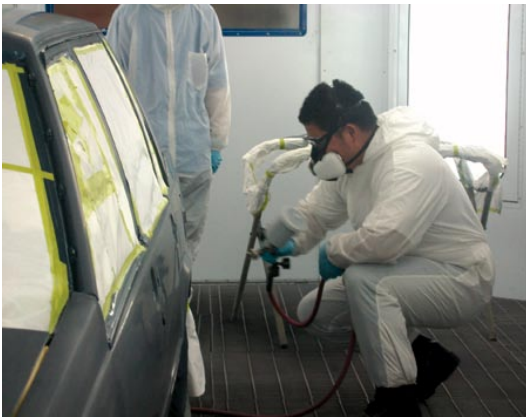
ABRP student outfitted with protective gear sprays paint in the painting booth.
